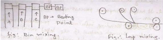
produced in the breaker scutcher. Four lap stands are placed before the finisher scutcher. For feeding four laps. Therefore, mixing can be done different ratio, like, 1/3; 1/1; 3/1;  $1/_{1/2}$ ;  $2/_{1/1}$  or 1/1/1/1 etc. This method is still used successfully.
