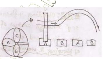
from the bales into the duct for mixing. For example, unimix of Reiter.
